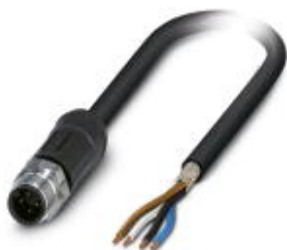
Sensor/Actuator cable, 4-position, PE-X/PE-X halogen-free, black-gray RAL 7021, shielded, Plug straight M12, A-coded, on free cable end, Cable length: 5 m, for outdoor applications, With high-grade steel knurl
