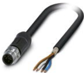
Sensor/Actuator cable, 4-position, PE-X/PE-X halogen-free, black-gray RAL 7021, shielded, Plug straight M12, A-coded, on free cable end, Cable length: 2 m, for outdoor applications, With high-grade steel knurl
