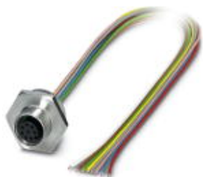
Sensor/actuator flush-type socket, 8-pos., M12, A-coded, front/screw mounting with M20 x 1.5 thread, with 0.5 m TPE litz wire, 5 x 0.34 mm 2 , high-grade steel version
