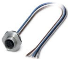
Sensor/actuator flush-type socket, 5-pos., M12, B-coded, front/screw mounting with M20 x 1.5 thread, with 0.5 m TPE litz wire, 5 x 0.34 mm 2 , high-grade steel version
