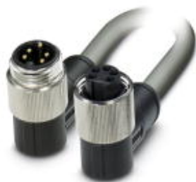
Power cable, 5-position, PUR, gray RAL 7001, Plug angled 7/8"-16UNF, on Socket angled 7/8"-16UNF, Cable length: 1 m, 1.5 mm 2 conductor cross section, For power supply
