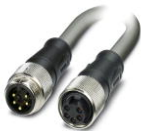
Power cable, 5-position, PVC, gray RAL 7001, Plug straight 7/8"-16UNF, A-coded, on Socket straight 7/8"-16UNF, A-coded, Cable length: 2 m, 1.5 mm 2 conductor cross section, For power supply
