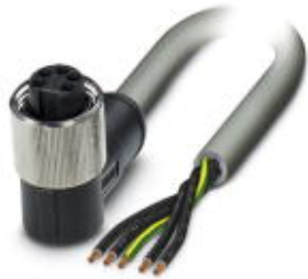
Power cable, 5-position, PVC, gray RAL 7001, free cable end, on Socket angled 7/8"-16UNF, Cable length: 7.5 m, 1.5 mm 2 conductor cross section, For power supply
