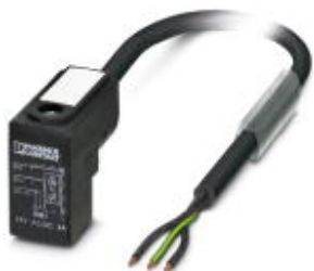
Sensor/Actuator cable, 3-position, PUR halogen-free, black-gray RAL 7021, free cable end, on Valve connector CI (9.4 mm), with 1 LED, connected with Varistor, Cable length: 3 m
