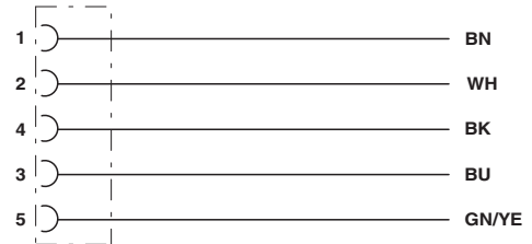
Contact assignment of the M12 sockets
