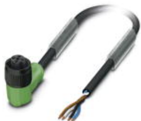
Sensor/Actuator cable, 4-position, PUR halogen-free, black-gray RAL 7021, free cable end, on Socket angled M12, A-coded, Cable length: 10 m, with plastic knurl
