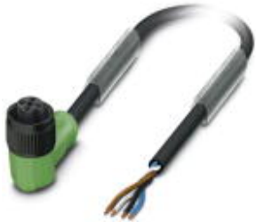
Sensor/Actuator cable, 4-position, PUR halogen-free, black-gray RAL 7021, free cable end, on Socket angled M12, A-coded, Cable length: 5 m, with plastic knurl
