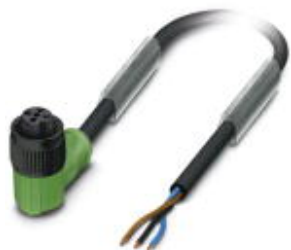
Sensor/Actuator cable, 3-position, PUR halogen-free, black-gray RAL 7021, free cable end, on Socket angled M12, A-coded, Cable length: 3 m, with plastic knurl
