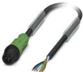
Sensor/Actuator cable, 5-position, PUR halogen-free, black-gray RAL 7021, Plug straight M12, A-coded, on free cable end, Cable length: 3 m, with plastic knurl
