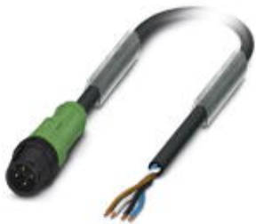
Sensor/Actuator cable, 4-position, PUR halogen-free, black-gray RAL 7021, Plug straight M12, A-coded, on free cable end, Cable length: 10 m, with plastic knurl
