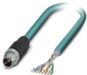
Assembled Ethernet cable, CAT6 A , shielded, 4-pair, AWG 26 stranded (7-wire), RAL 5021 (water blue), M12 plug on free conductor end, length 2 m
