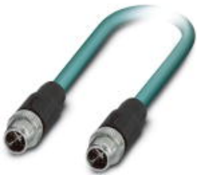
Assembled Ethernet cable, CAT6 A , shielded, 4-pair, AWG 26 stranded (7-wire), RAL 5021 (water blue), M12 plug on M12 plug, length 1 m
