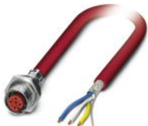
Bus system flush-type socket, CC-Link, 4-pos., M12, SPEEDCON, shielded, rear/screw mounting with Pg9 thread, with 2.0 m bus cable
