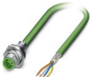
Bus system flush-type plug, PROFINET, 4-pos., M12, shielded, D-coded, SPEEDCON, rear/screw mounting with Pg9 thread, with 0.5 m bus cable, 2 x 2 x 0.34 mm 2
