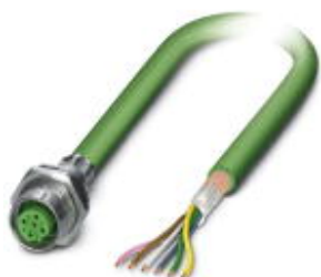
Bus system flush-type socket, INTERBUS, 5-pos., M12, shielded, B-coded, SPEEDCON, rear/screw mounting with Pg9 thread, with 1.0 m bus cable, 3 x 2 x 0.25 mm 2
