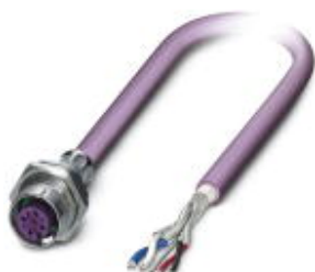
Bus system flush-type socket, DeviceNet/CANopen, 5-pos., M12, shielded, A-coded, Speedcon, rear/screw mounting with Pg9 thread, with 2.0 m bus cable, 2 x 0.2 mm 2 ; 2 x 0.32 mm 2
