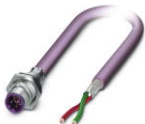
Bus system flush-type plug, PROFIBUS, 2-pos., M12, shielded, B-coded, SPEEDCON, rear/screw mounting with Pg9 thread, with 0.5 m bus cable, 2 x 0.25 mm 2
