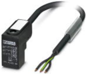
Sensor/Actuator cable, 3-position, PUR halogen-free, black-gray RAL 7021, free cable end, on Valve connector CI (9.4 mm), with 1 LED, connected with Z diode, Cable length: 5 m
