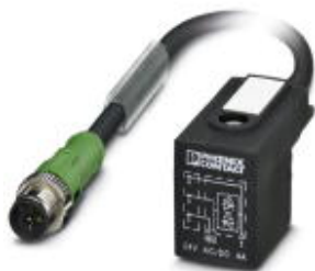
Sensor/Actuator cable, 3-position, PUR halogen-free, black-gray RAL 7021, Plug straight M12 SPEEDCON, A-coded, on Valve connector B (10 mm), with 1 LED, connected with Z diode, Cable length: 1.5 m
