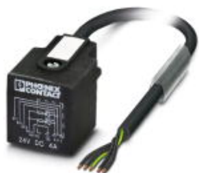
Sensor/Actuator cable, 5-position, PUR halogen-free, black RAL 9005, free cable end, on Valve connector AD (pressure switch), with 2 LEDs, Cable length: 5 m
