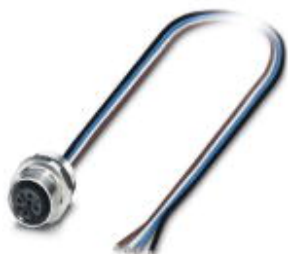
Bus system flush-type connector, FOUNDATION Fieldbus, socket, 4-pos., M12, A-coded, front/screw mounting with Pg9 thread, with 0.5 m TPE litz wire, 3 x 0.34 mm 2 , stainless steel version
