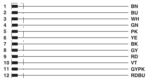
Contact assignment of the M12 plug
