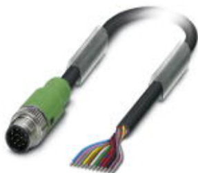
Sensor/Actuator cable, 12-position, PUR halogen-free, black RAL 9005, Plug straight M12 SPEEDCON, A-coded, on free cable end, Cable length: 1.5 m
