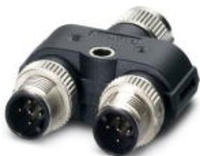
Y distributor, 5-position, shielded, Socket straight M12 SPEEDCON, A-coded, on Plug straight M12 SPEEDCON, A-coded and Plug straight M12 SPEEDCON, A-coded, Parallel distributor
