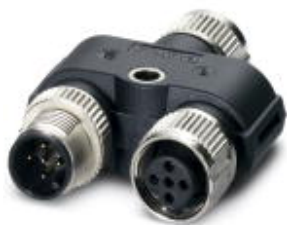
Y distributor, 5-position, shielded, Socket straight M12 SPEEDCON, A-coded, on Socket straight M12 SPEEDCON, A-coded and Plug straight M12 SPEEDCON, A-coded, Parallel distributor
