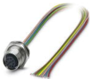
Sensor/actuator flush-type socket, 8-pos., M12 SPEEDCON, rear/screw mounting with M16 thread, with 0.5 m TPE litz wire, 8 x 0.25 mm 2
