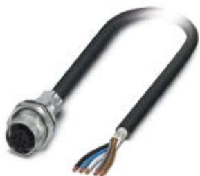
Flush-type socket, shielded, 5-pos., M12, A-coded, rear/screw mounting with M16 thread, with 1 m line, 5 x 0.34 mm 2
