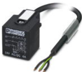
Sensor/Actuator cable, 3-position, PVC, black RAL 9005, free cable end, on Valve connector A, with 1 LED, connected with Z diode, Cable length: 3 m
