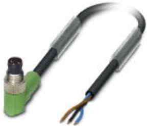
Sensor/Actuator cable, 3-position, PVC, black RAL 9005, Plug angled M8, on free cable end, Cable length: 1.5 m
