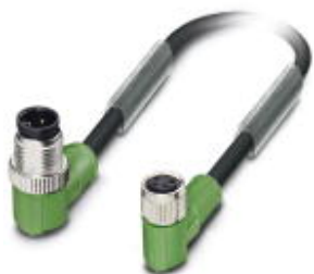
Sensor/Actuator cable, 4-position, PVC, black RAL 9005, Plug angled M12, A-coded, on Socket angled M8, Cable length: 0.6 m
