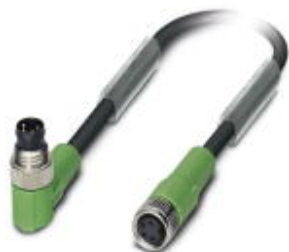
Sensor/Actuator cable, 4-position, PVC, black RAL 9005, Plug angled M8, on Socket straight M8, Cable length: 1.5 m
