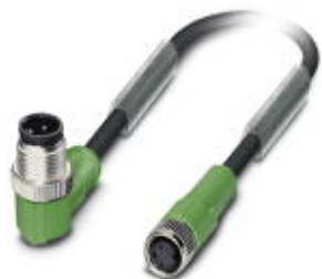
Sensor/Actuator cable, 3-position, PVC, black RAL 9005, Plug angled M12, A-coded, on Socket straight M8, Cable length: 0.3 m
