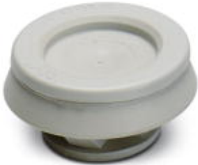
Membrane screw connection, Cable gland material: Polypropylene, Application: Standard, External cable diameter 9 mm ... 17 mm, Shielding: No, Connecting thread: M25, Color: lightgrey RAL 7035
