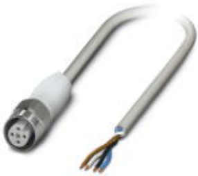
Sensor/Actuator cable, 4-position, PP-EPDM halogen-free, gray RAL 7035, free cable end, on Socket straight M12, A-coded, Cable length: 3 m, Hygienic design, With high-grade steel knurl
