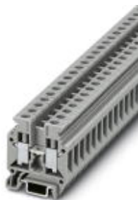
Mini feed-through terminal block, Connection method: Screw connection, Cross section: 0.2 mm 2 - 6 mm 2 , AWG: 24 - 10, Width: 6.2 mm, Color: gray, Mounting type: NS 15
