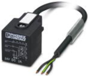
Sensor/Actuator cable, 3-position, PUR halogen-free, black-gray RAL 7021, free cable end, on Valve connector A, with 1 LED, connected with Damping diode, Cable length: 10 m
