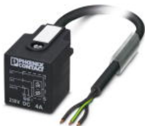
Sensor/Actuator cable, 3-position, PUR halogen-free, black-gray RAL 7021, free cable end, on Valve connector A, with 1 LED, connected with Varistor, Cable length: 3 m
