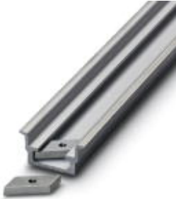
Slide nut, for DIN rail NS 35/15-AL, with M4 thread, for mounting equipment, material: Steel
