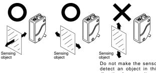
Do not make the sensor detect an object in this direction because it may cause unstable operation.
