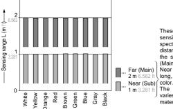
These bars indicate the sensing range with respective colors when the distance adjuster is set at the sensing range of Far (Main) 2 m ft and Near (Sub) 1 m 3 long, each, with white
