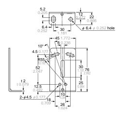
Material: Cold rolled carbon steel (SPCC) Two M4 (length 25 mm 0.984 in) screws with washers and two M4 nuts are attached.
