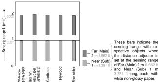
sensing range with spective objects when the distance adjuster is set at the sensing range of Far (Main) 2 m 6.562 ft and Near (Sub) 1 m ft long, each, with white non-glossy paper.
