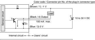
Symbols ... D : Reverse supply polarity protection diode  $$\sf Z{\it D}$$  : Surge absorption zener diode Tr: NPN output transistor
