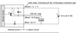
Symbols ... D : Reverse supply polarity protection diode ZD: Surge absorption zener diode Tr: PNP output transistor
