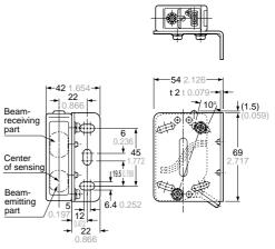
DIMENSIONS (Unit: mm in) The CAD data in the dimensions can be downloaded from the SUNX website: http://www.sunx.co.jp/
