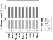
These bars indicate the sensing range with the respective colors when the distance adjuster is set at the sensing range of 2 m 6.562 ft, 1 m 3.281 ft and 0.2 m 0.656 ft long, each, with white color.
