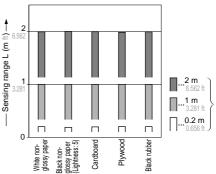
These bars indicate the sensing range with respective objects when the distance adjuster is set at the sensing range of 2 m 6.562 ft, 1 m 3.281 ft and 0.2 m 0.656 ft long, each, white non-glossy paper.
