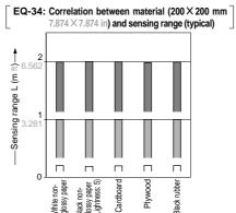
These bars indicate the sensing range with the respective objects when the distance adjuster is set at the sensing range of 2 m 6.562 ft, 1 m 3.281 ft and 0.2 m 0.656 ft long, each, with white non-... 0.2 m glossy paper.
