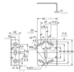
Material: Cold rolled carbon steel (SPCC)
