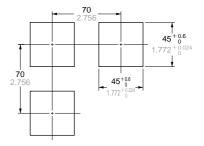
Note: The panel thickness should be 1 to 3.2 mm 0.039 to 0.126 in.
