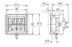
portion shows the front protection cover. Material: Polycarbonate (Front protection cover) Nylon 6, Polyacetal (Panel mounting bracket)
