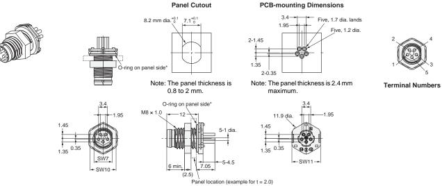
\*The O-ring on the panel side maintains a waterproof structure (IP67) between the panel and Connector.
