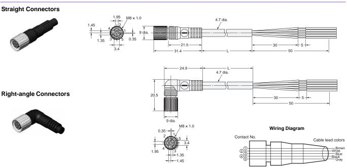
S8 Snap-in Connectors with Vibration-proof Robot Cable
