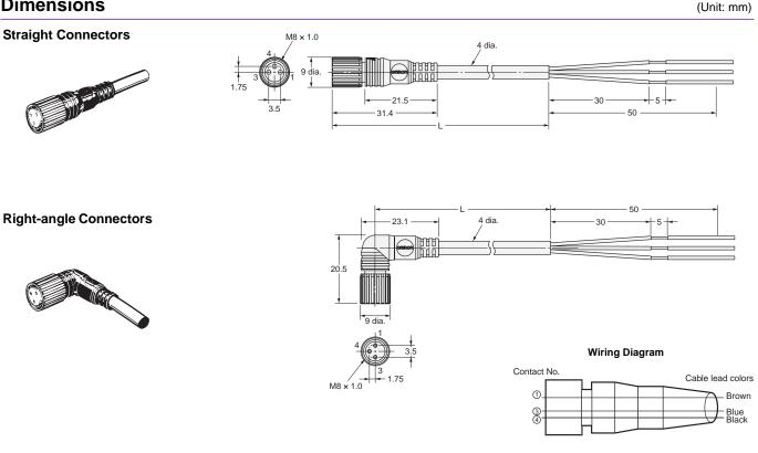
M8 4 pin Screw-on Cables with Vibration-proof Robot Cable/Standard Cable
