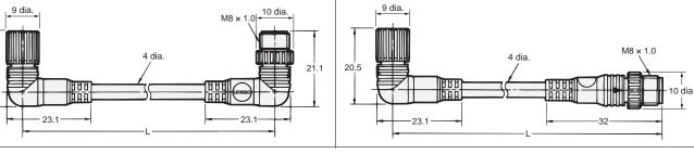
S8 Snap-in Connectors with Vibration-proof Robot Cable
