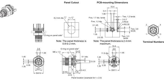
\*The O-ring on the panel side maintains a waterproof structure (IP67) between the panel and Connector.
