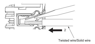
Remove the flat-blade screwdriver from the release hole.
