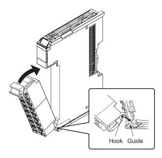
Mount a Terminal Block that is applicable to each Unit model.
