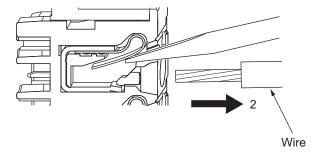
Remove the flat-blade screwdriver from the release hole.
