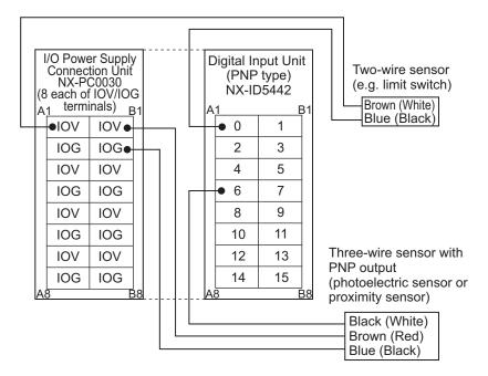
Note Connecting three-wire sensors to all 16 inputs requires two NX-PC0030 Units.
