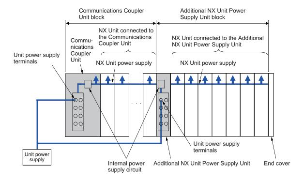
The total Unit power supply capacity for these two blocks is the power supply capacity that the Slave Terminal requires.
