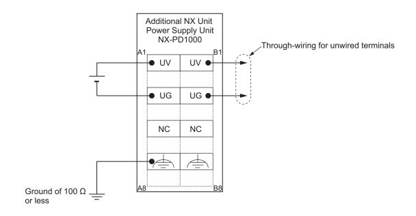
Ground the functional ground terminal to 100  $\Omega$  or less.
