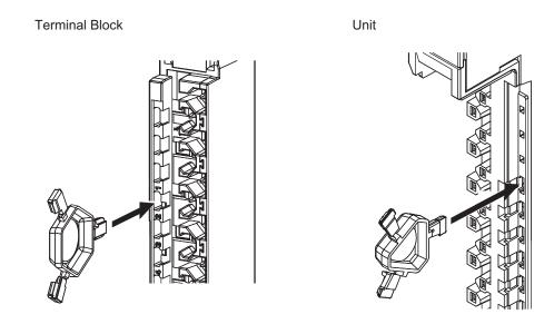
2 Rotate the runner to break off the Coding Pin.
