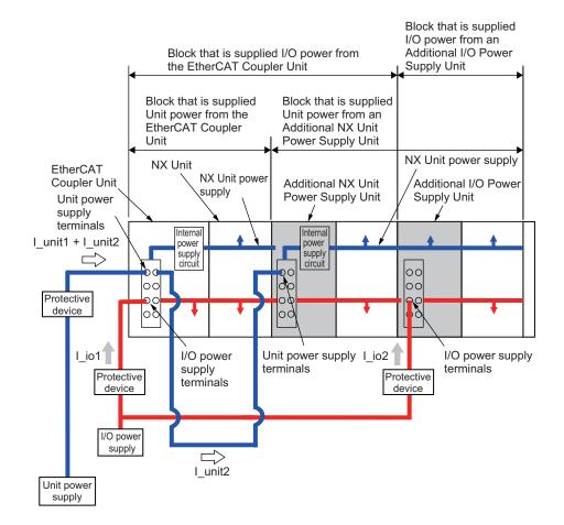
When total current consumption for all blocks does not exceed the rated current
