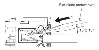
Leave the flat-blade screwdriver pressed into the release hole and pull out the wire.
