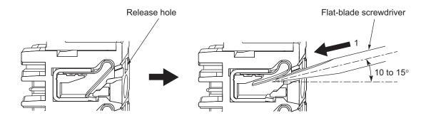
Leave the flat-blade screwdriver pressed into the release hole and insert the twisted wire or the solid wire into the terminal hole.
