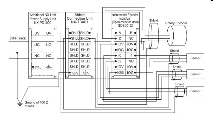
Connect the shield of cable to the SHLD terminal.
