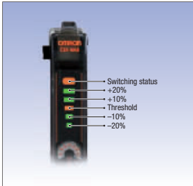
Bargraph display with light level, switching status and threshold indicators
