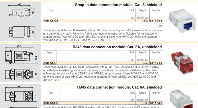
Connection module Cat. 6A (ISO) shielded, with a RJ45 slot. Including an EMC screen hood, a dust cover, a cable tie, a Keystone fastening frame and mounting instructions. Suitable for installation in the data technology supports of type DTG-2C and DTS-2C, support plate of type MTM 2C and MTM 3C, mounting plate of type MPR2 2C, mounting supports of type MTGE2 2C, MTGE2 15 2C and MTGE2 F 2C.
