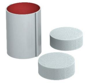
Internally coated pipe shells with click lock. The inner space can be fitted with cables and electrical installation pipes completely. Approved in Europe with ETA-13/0904. Fire resistance classes to EI120.
