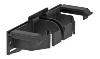
Cover adapter for mounting on duct bases and fittings of the GAD design device installation duct series. The cover adapter can be pushed into a guide on the base and is used to accept the duct cover and keep it at the desired spacing. It is also used for bundled cable exits and can be moved into the lengthwise direction. A maximum spacing of 50 cm between the cover adapters must be maintained.
